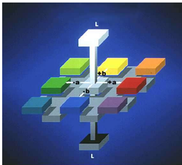
Fig. 4: Measurement of colour according to ISO 7724 (DIN 5033).
