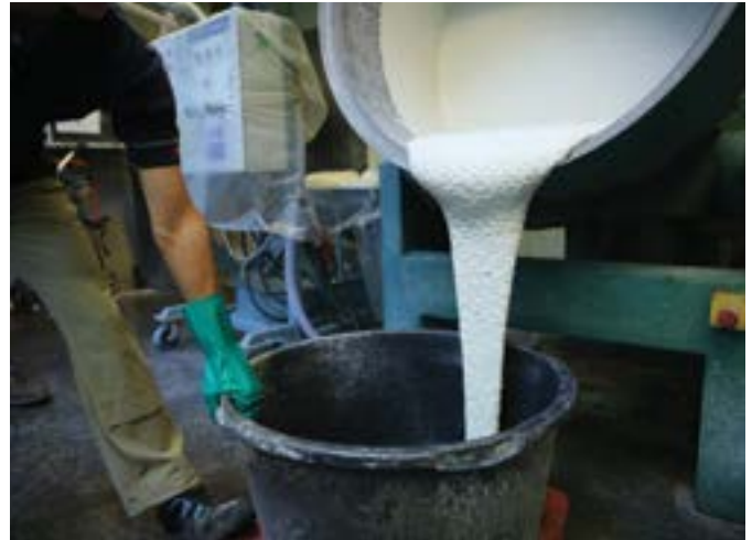
A batch of AALBORG EXTREME Light 120 is discharged from a laboratory pan mixer. The prepackaged material exhibits excellent stability and a slump flow of 900 mm (35 in.)
